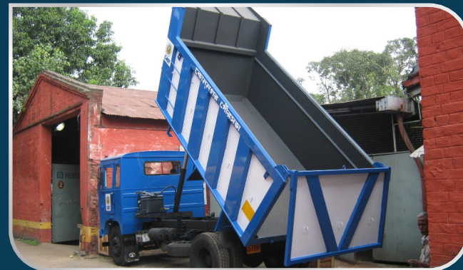
Box Type Tipper Body (Front End Tipper Body) using HYVA Hydraulic Kit
