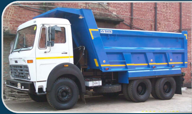
Box Type Tipper Body (Front End Tipper Body) using HYVA Hydraulic Kit (14CuMt. - 28CuMt.)
