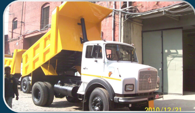
Sandwiched Scow Body (Front End Tipper Body) With Rock Breaker using HYVA Hydraulic Kit
