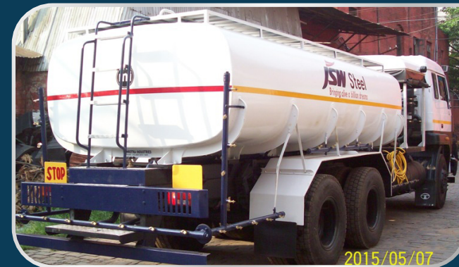
WATER SPRINKLER / Dust Suppression System
